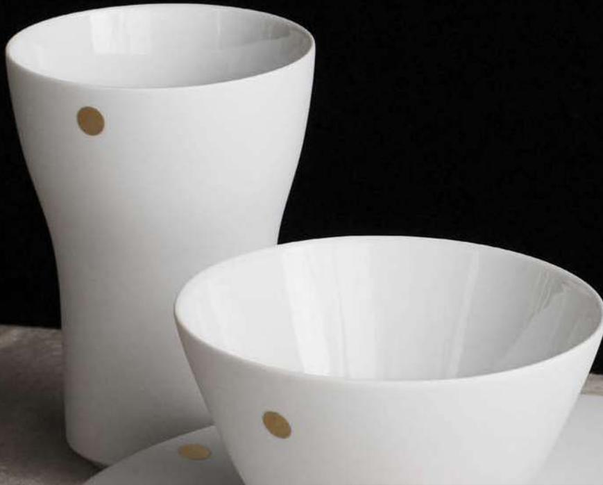
The circles of the decor are created with real gold, which is processed in a paste in a multilayer ceramic silkscreen print. The resulting serigraphy is applied by hand to the high-fired porcelain with a transfer medium and fuses in a final firing at 810-830°C.
