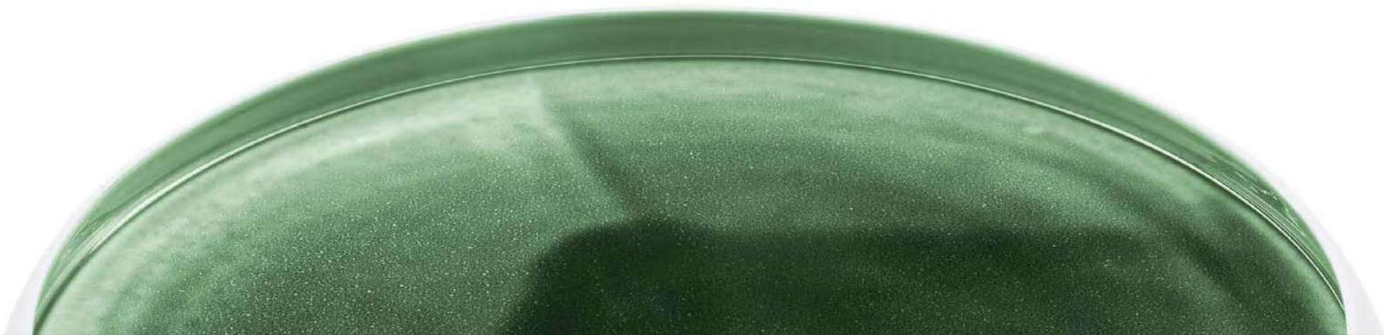
An additional glaze made of a mixture of chromium oxide and other metal oxides is applied to already glazed surfaces of the porcelain, which fuse with the clear glaze in a second high-fire. The complex process ensures strong adhesion of the glaze and thus durability and longevity. Due to various chemical reactions and formations of the raw colorants, Emerald Green alternates with a lighter, almost translucent hue, making each piece of Emerald unique.
