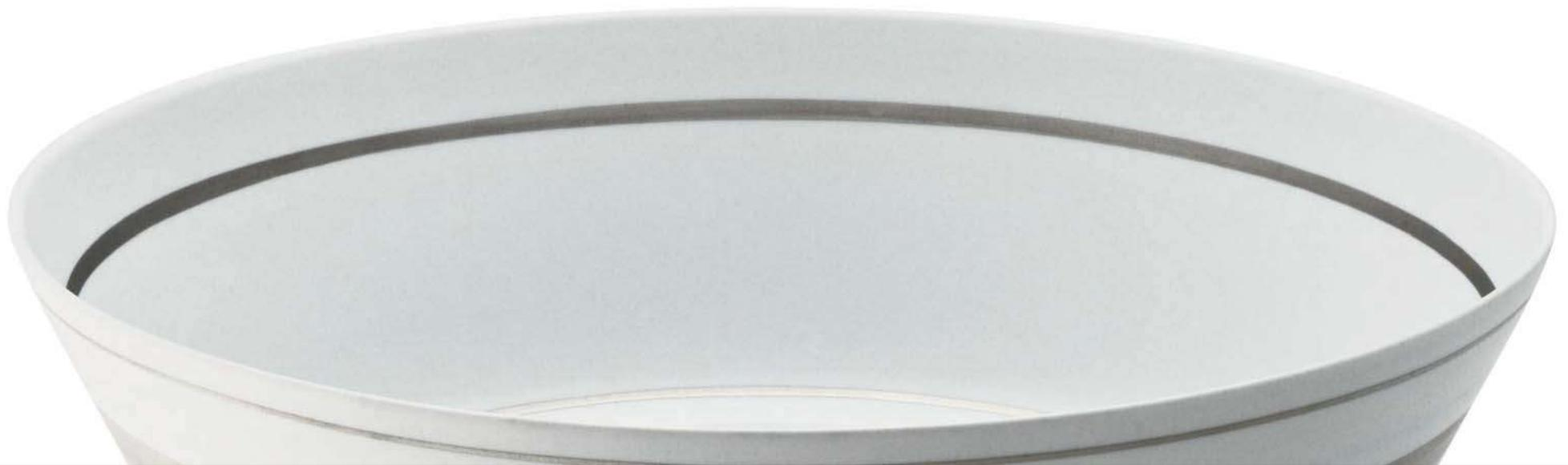
To guarantee the adhesion of the precious metal, the smoothly fired porcelain is polished and cleaned before application. Then, genuine platinum is hand-painted in narrow and wide circles that fuse with the glazed porcelain during an additional firing. A final polishing of the precious metal surface unfolds the silky-matt sheen characteristic of the decor.
