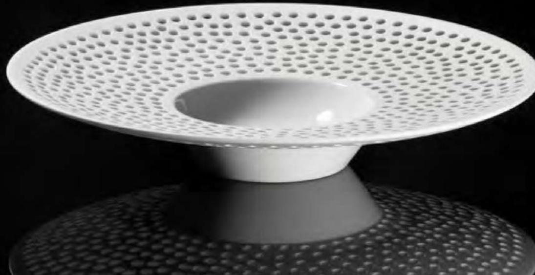
Cielo is undoubtedly our most elaborate decoration: each hole is drilled individually and by hand into the leather-hard, unfired porcelain. The holes are then plastered with a sharp stainless steel blade and smoothed with a fine sponge.
